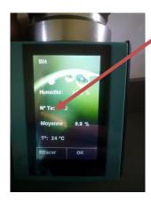
"N° Te: 2" indicates the number of successive measurements you have made. In this example there are 2 measurements. It is the result of the last measurement that is displayed, together with the average of the 2 measurements and the sample temperature.
