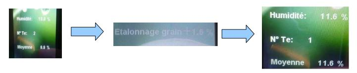
The purpose of calibration is to obtain results set to your Storage Agency's appliance. When applying a bias with a storage agency, use a homogeneous, stable and mature grain sample.
